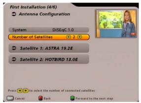
Use the **()** buttons to select how many satellites (max. 4) you would like to receive with your reception system. The following display appears (example):
